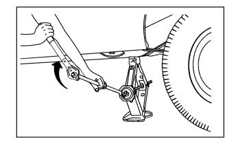
4. Raise the vehicle by turning the ratchet clockwise. Make sure the UP mark faces you. Raise the vehicle far enough off the ground so there is enough room for the spare tire to fit.
